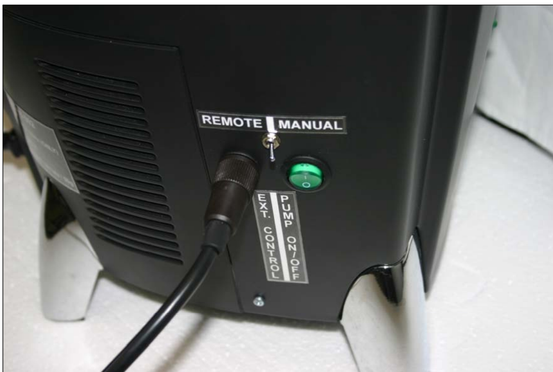
Fig.17: Pump switch; remote / manual switch
