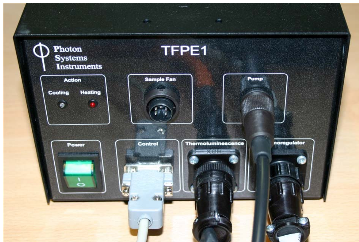
Fig.9: TFPE1 Control System – front panel with connectors
