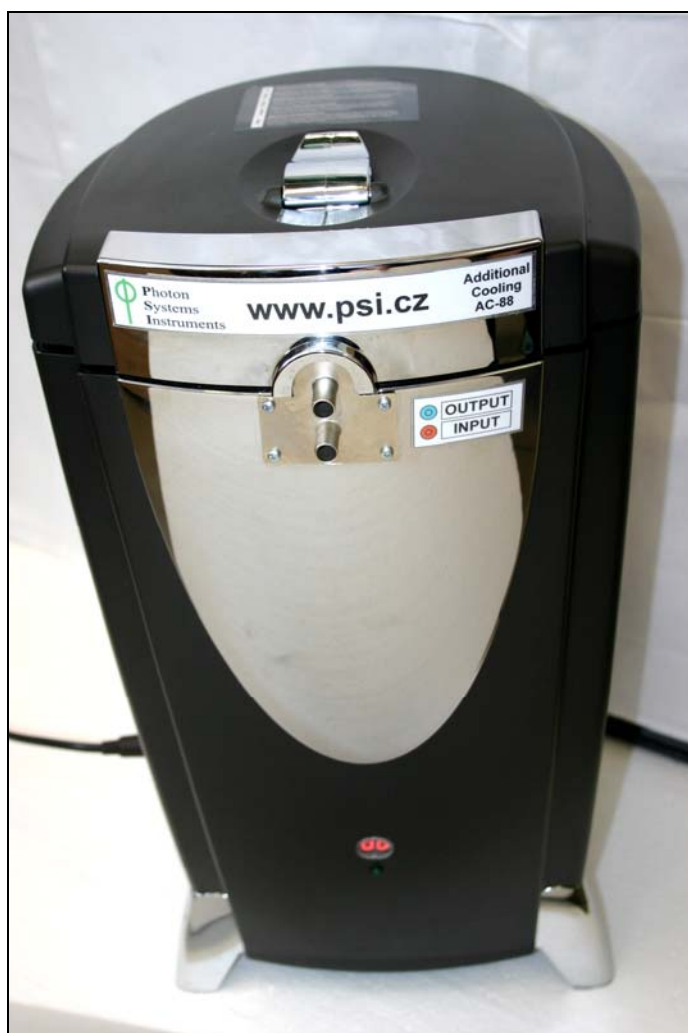
Fig.12: AC-88 Water Cooling Unit – front view
