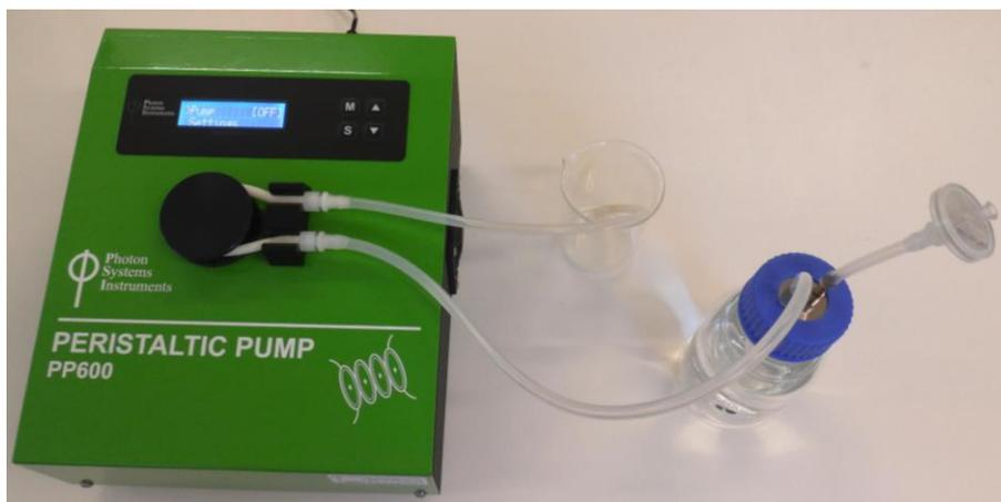
Fig. 6 Basic configuration of Peristaltic Pump.
