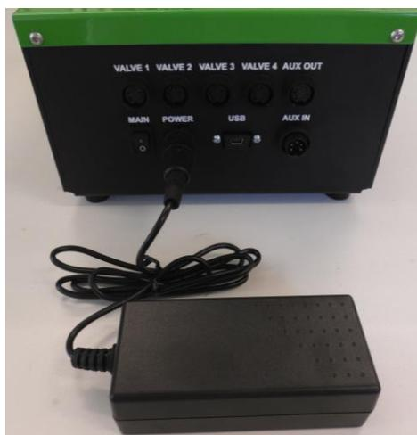
Fig. 7 Power cord connection of peristaltic pump.
