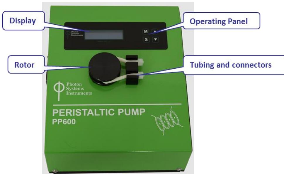
Fig. 3 Front panel.
